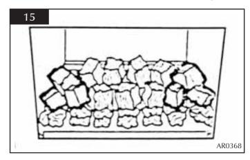
6.12 Place five small coals along the rear of the flame baffle, resting against the rear ledge, see diagram 16.
